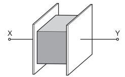
The cube has volume V and is made of a material with resistivity  $\rho$ . The connections to the cube have negligible resistance.
