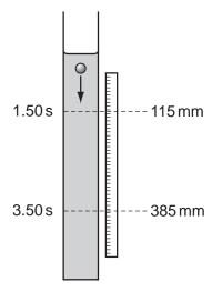
There are two marks on the tube. The top mark is positioned at 115  $\pm$  1 mm on the adjacent rule and the lower mark at 385  $\pm$  1 mm. The ball passes the top mark at 1.50  $\pm$  0.02 s and passes the lower mark at 3.50  $\pm$  0.02 s.
