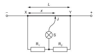
To determine the ratio  $\frac{V_1}{V_2}$  of the potential differences across  $R_1$  and  $R_2$ , a point is found on XY at which the lamp is off. This point is at a distance *x* from X.
